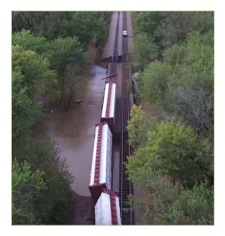
Figure 16: Derailment of BNSF train from washout of bridge over Rush Creek south of Ferryville, WI, September 22, 2016. *Source:* Snapshot from YouTube video, DOT-111.info.
