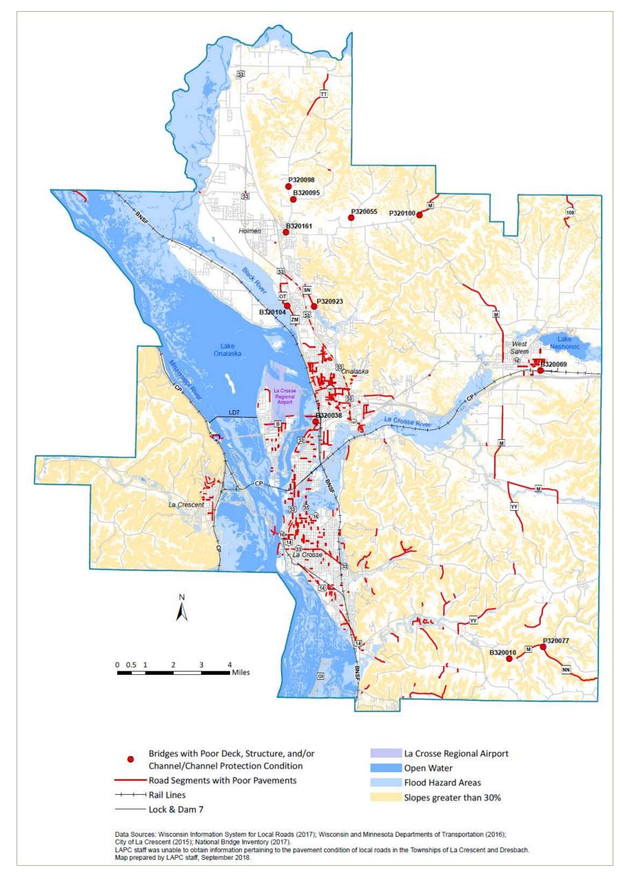
Figure 17: Road structures and pavements in "poor" condition.
