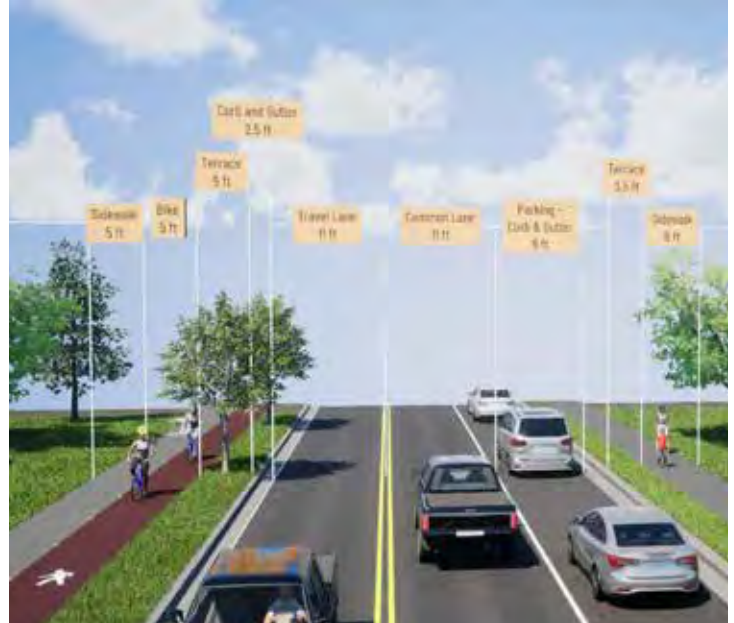
N 4th St to Park St
