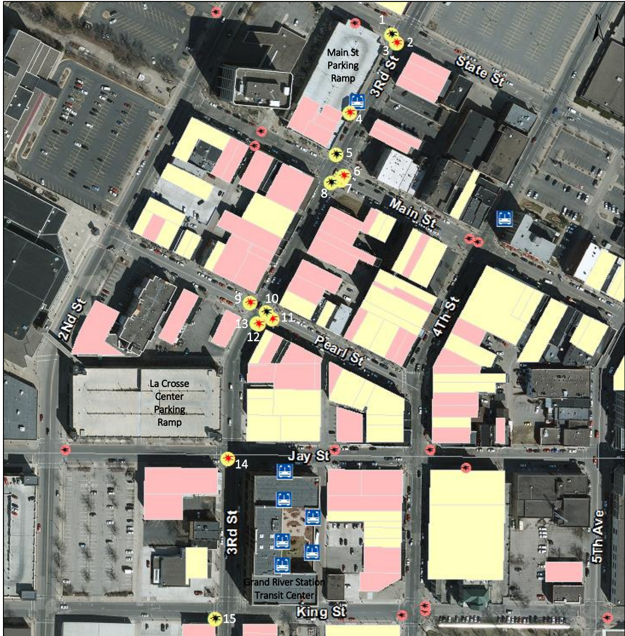
Figure 30: Bicycle and pedestrian crashes along the 3 rd St corridor between State St and King St, 2011-2015. The figure illustrates the bicycle (black/yellow) and pedestrian (red/yellow) crashes, other crashes that are not along the corridor (pink/black), MTU bus stops (bus symbols), and the most popular land uses along and near the corridor. Eating and drinking establishments are in pink and retail and service establishments are in yellow. The crash location numbers correspond to the crash numbers in Table 13.
