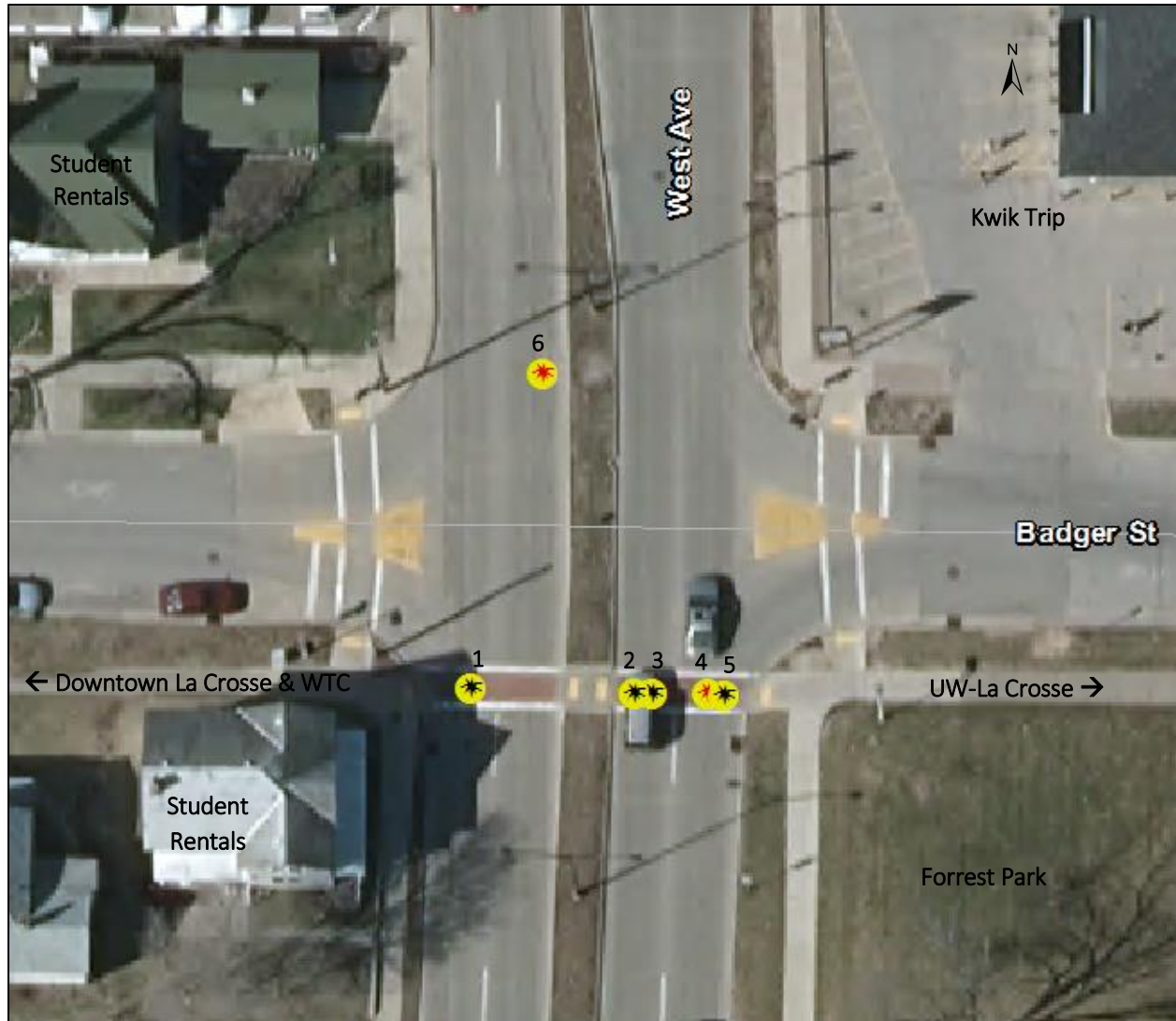
Figure 23: Bicycle and pedestrian crashes at the West Ave/Badger St intersection, 2011-2015. Yellow/black symbols represent bicycle crashes and yellow/red symbols represent pedestrian crashes. The crash location numbers correspond to the crash numbers in Table 8.
